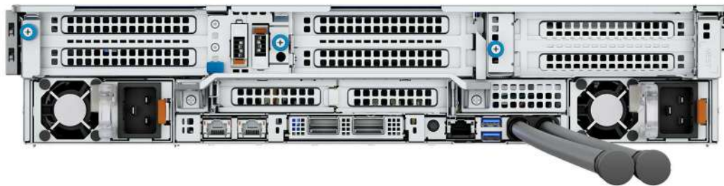
Figure 6. Rear view of the system with optional liquid cooling
