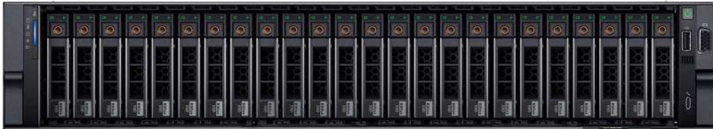
Figure 1. Front view of 24 x 2.5-inch drive system
